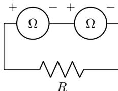
$$R = R_{\Omega 1} + R_{\Omega 2} = 1507 \text{ кОм} + 1510 \text{ кОм} = 3017 \text{ кОм} \approx 3020 \text{ кОм}.$$
